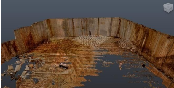
Figure 3.4.1 Obtained Point Cloud resulting from the connection of obtained individual scans – front view
