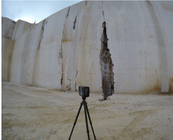
Figure 2.5.2 FARO laser scanner in operation, author photo
