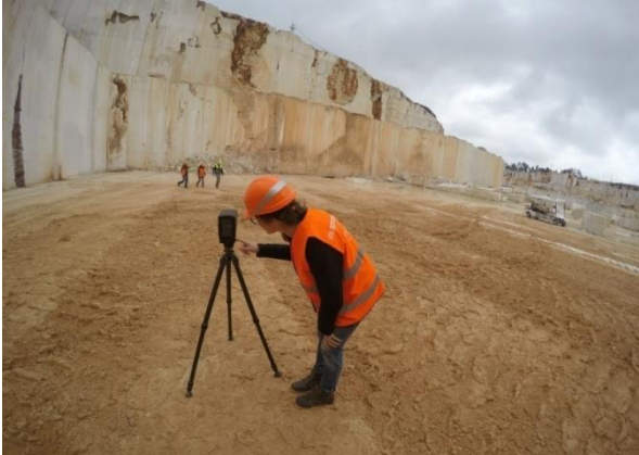
Figure 3.3.2 Setting up the laser scanner
